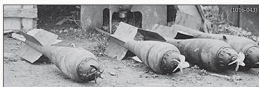
20lb Cooper bombs as carried by 148th Aero Sqn Camels on ground attack duties.
