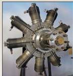
^ 160hp Gnome 9N Monosoupape on display at The Vintage Aviator LTD.
