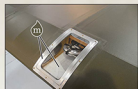
Aileron control cable pulley inspection door from the starboard bottom wing of B5663. This was usually overpainted in late serving aircraft.
