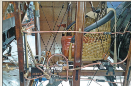
Interior fuselage detail from Sopwith F.1 Camel B5663 nearing completion of its restoration to flying status at The Vintage Aviator Ltd (TVAL) in late 2014. Note the 4 point safety harness which is almost never seen on WW1 era Camels.
